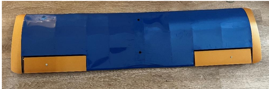
FIGURE 27: MANUFACTURED MAIN WING
