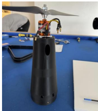
FIGURE 6: 3-D printed nose cone
