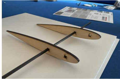
FIGURE 5: Balsa wood ribs and carbon fiber spars
